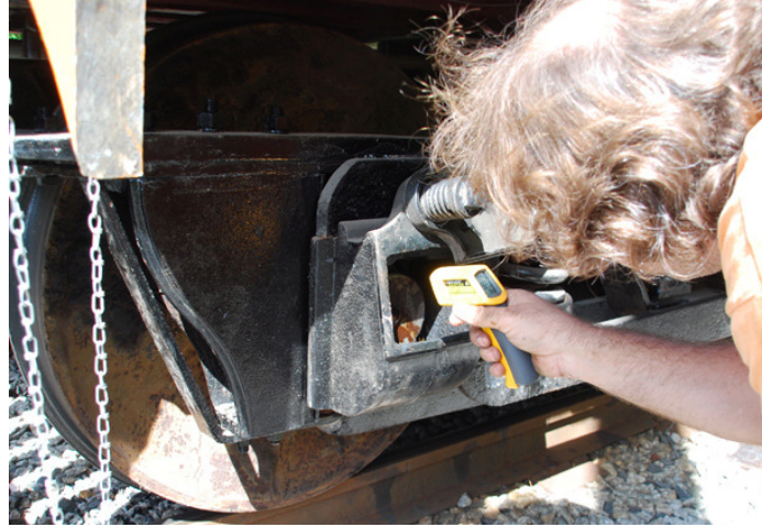
Randy taking temperature of the journal bearing that had overheated on a previous trip
