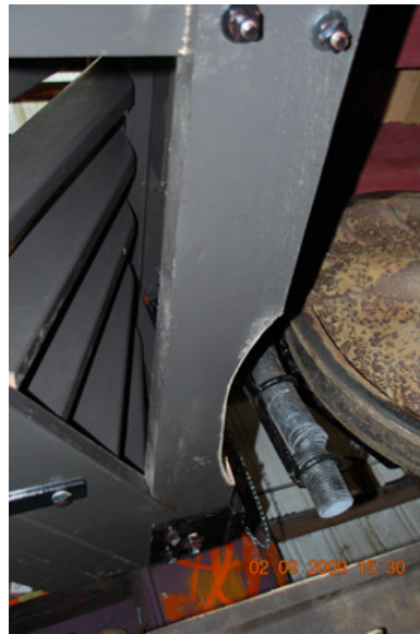
Cut-away area under pilot brace to clear the sander
